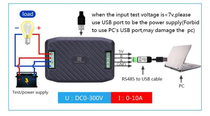
1 RS485 interface is passive output, need external connect 5V power supply and the the external power supply should >100mA
