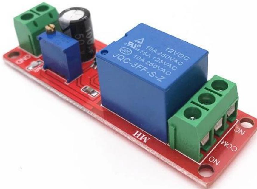
1. power relay delay pull. Specifically: 12v power supply to the relay, the relay will not immediately suck and status relay outputs are normally open disconnected public, normally closed and public conduction, wait until the delay 1-10s (adjustable), the relay suction and, this time, the relay output status is: normally open and public conduction, normally closed and public disconnected; as long as uninterruptible power module, this state will remain.
