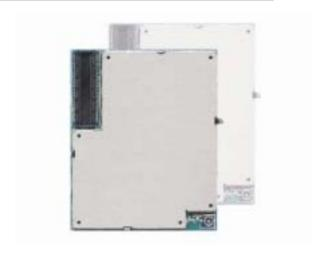
The SIM340 is a complete Quad-band GSM/GPRS solution in a compact plug-in module.
