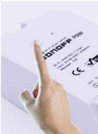
2. Press the button for 7 seconds until the green LED blinks like this: blinks 3 times and on repeatedly:
