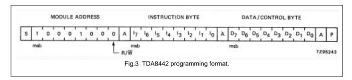
Acknowledge (A) is generated by the TDA8442 only when a valid address is received and the device is not in the power-down-reset mode ( $V_P > 8.5 \text{ V (typ.)}$ ).
