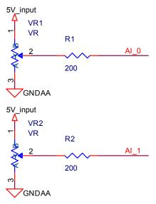
Figure 7. Variable Resistor Circuit of the WIZ220IO Base Board
