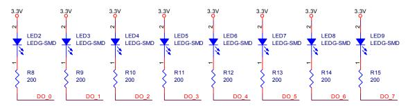
Figure 4. LED circuit of WIZ220IO Base Board
