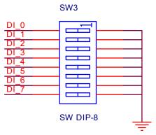
Figure 5. DI Switch of the WIZ220IO Base Board
